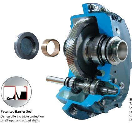
**AGMA Class 12 Gearing** and Tapered Roller Bearings Helical gearing is cut to AGMA Class 12 and keyed to all shafts. All shafts utilize tapered roller bearings.
